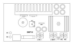
**Note:** SMP10 units are available completely assembled in an enclosure (15.5"H x 12"W x 4.5"D) with transformer and cam lock as the following model numbers: SMP-10C12X for 12 VDC output, SMP-10C24X for 24VDC output.
